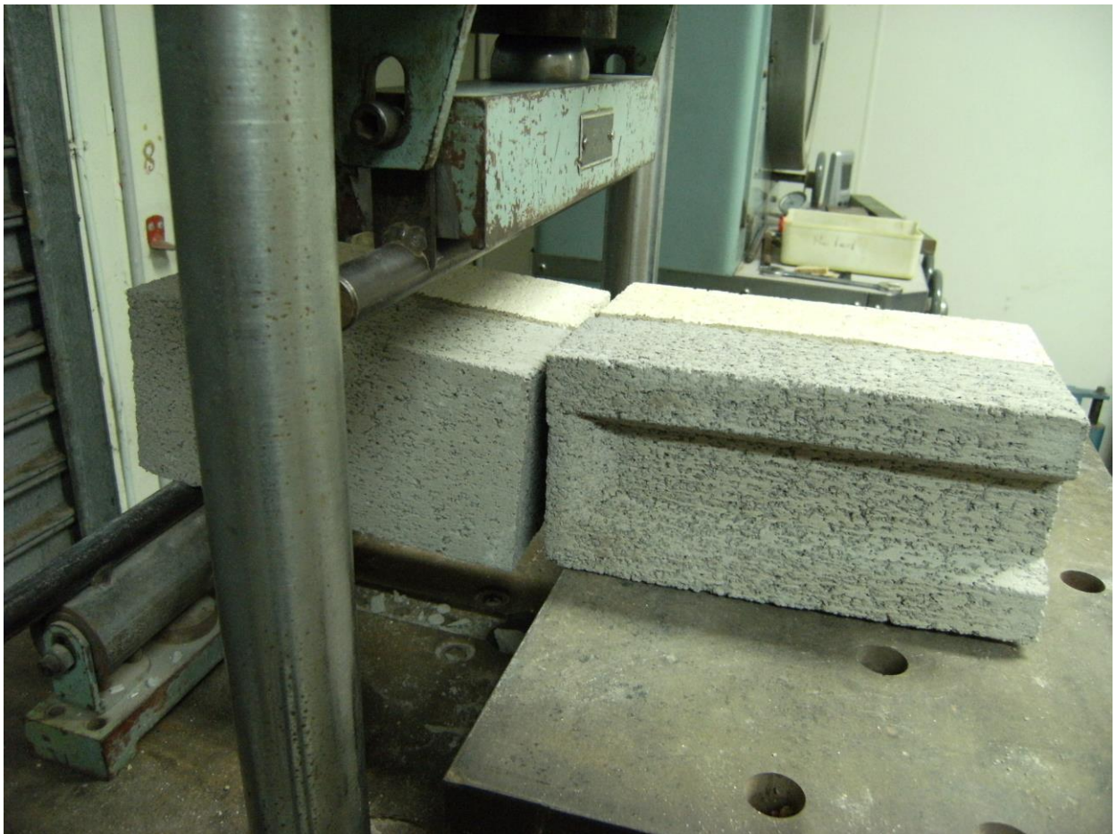
One of the specimens after testing. Each end of the tie was embedded in mortar (1 cement : 1 lime : 6 cement) between two bricks, with a spacing of 10mm between the couplets. One couplet was clamped to the testing machine (right of photo; clamps not shown). The other was supported 25mm in from the end. The load was applied to the left couplet, 25mm from the central spacing.
