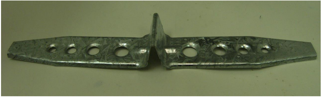
One of the expansion ties
