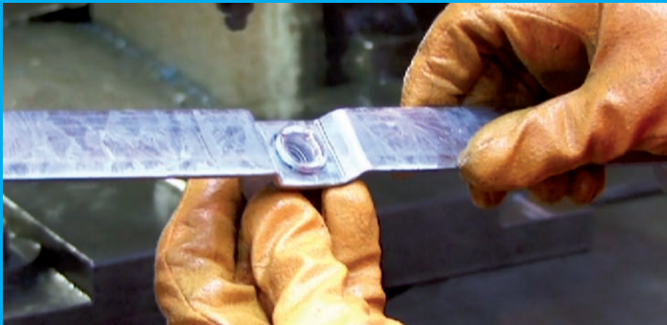
Abey's manufacturing facility showing press stamping of components that is stronger and less corrosive than welding.
